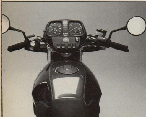
*The K75's instruments and warning lights are neat and easily readable. Those rockers below the ignition switch are dummies that can be replaced with real switches when accessories are added.*
